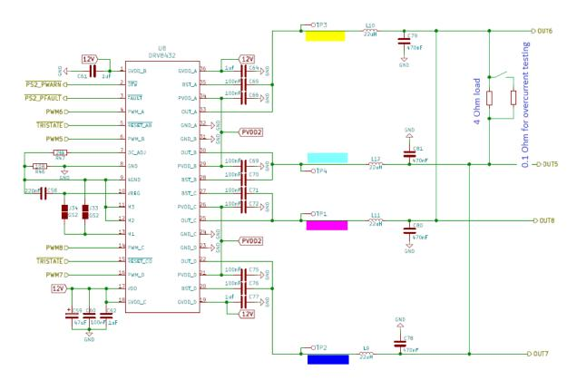
The ~FAULT is asserted LOW when one or more half-bridges are detecting OCP. The other half-bridges in the same IC will still operate normally; the ones which had an OCP will be in High-Z.
