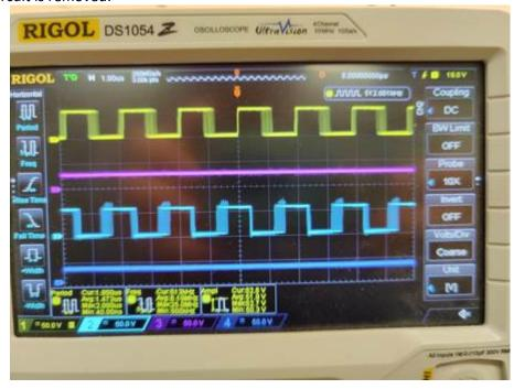
The yellow and magenta traces are signals on the first bridge PWM outputs. The cyan and blue traces are signals on the second bridge PWM outputs. Load is connected after the filter inductors.
