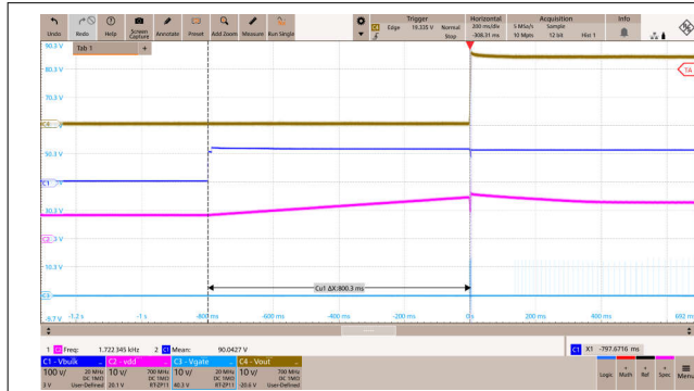
Figure 8-4. Start-Up Waveforms at 85Vac and No Load
