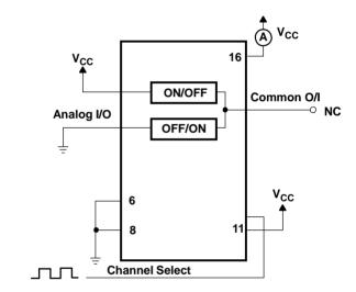
Figure 15. Power-Dissipation Capacitance Test Setup
