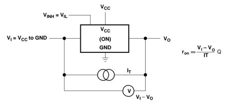
Figure 5. On-State-Resistance Test Circuit
