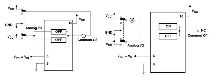
Figure 7. Maximum Off-Channel Leakage Current, Common Channel, Test Setup
