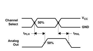
Figure 9. Propagation Delays, Channel Select to Analog Out
