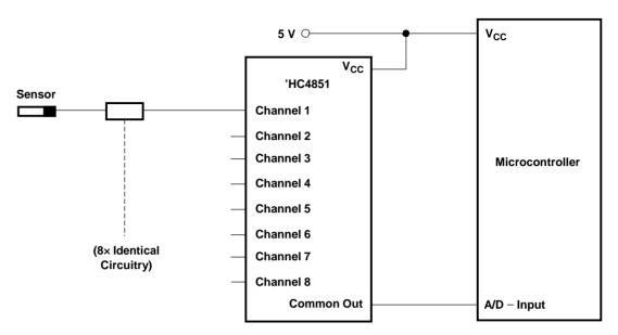
Figure 3. Solution by Applying the 'HC4851 Multiplexer
