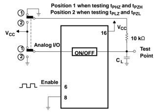
Figure 13. Propagation Delays, Enable to Analog Out
