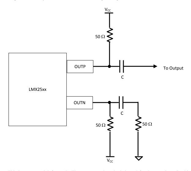
This is pretty straightforward. The output needs to be balanced for the negative. So this assumes the output is a 50 ohm load. If you are feeling adventurous, you could technically terminate the 50 ohm on OUTN to Vcc, but this has not been tried.
