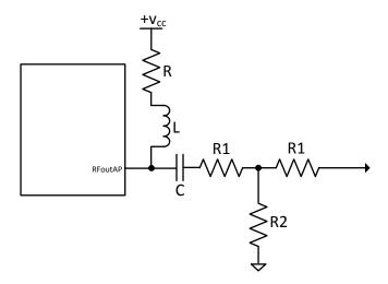
R is the pull-up resistor. In this case, 50 ohm might be a good choice, but maybe 25 ohm is a good choice at higher frequencies. Note that there are high frequency resistors available for both 50 and 25 ohm. For the inductor, 1 nH to 3 nH might be a reasonable choice. R1 and R2 form a resistive T pad. For the AC couping cap, C, one was put on the bottom of the pad instead of the junction of L and R1 in order to put less components in the high frequency path.
