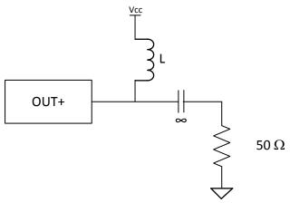
For the purposes of matching the inductor, one may think that there is an "optimal" value (assuming the output buffer to be high impedance) for the purposes of impedance matching. Nevertheless, it's good to through the exercise. Calculate the reflection coefficient.
