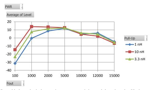
At 1 GHz and below, the inductor size matters, as it is much less than the 50 ohms. At 2 GHz, we see the 10 nH is getting lower, but we are also getting maybe too close to the self-resonant frequency for that. But we see higher power for the 1 and 3.3 nH inductors. At 5 GHz, the theoretical pull-up inductor impedance is high enough, but now we are near the point where the device output impedance is low. Beyond this, it seems that other effects dominate.
