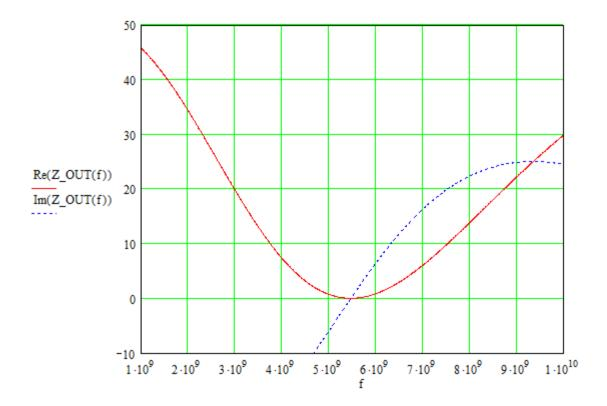
The thing to take not of specifically is that around Note around 5 GHz, impedance is theoretically low for this example using a 50 ohm pull-up. Note also that this is where  $C_{\text{INT}}$  resonates with  $L_{PKG}$ . So this low impedance is likely to be an issue for just about any pull-up at 5 GHz.
