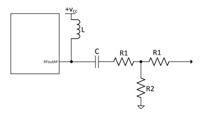
Here are some resistor values for common T pads:
