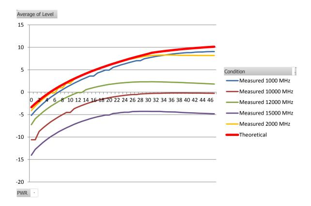
At 1000 MHz, the measured power is actually lower. This could be because the AC coupling capacitor was too small and there was some loss. At 2000 MHz, there is very good match up to PWR=30, but then we see saturation occurring earlier than predicted by the model. Then at 10,12, and 15 GHz, we see some saturation even earlier, possibly due the the Miller capacitance, which increases with PWR.
