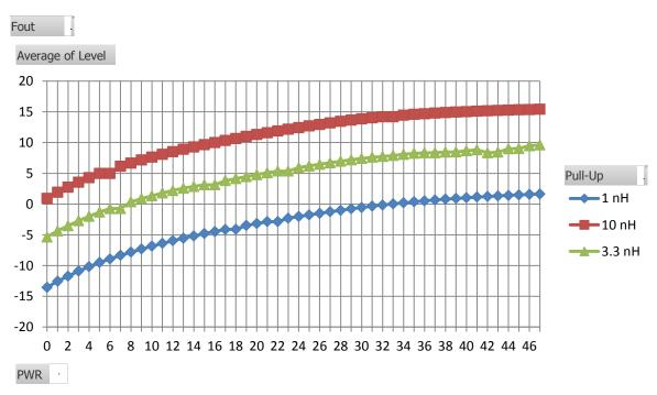
Now if we look at 1 GHz and sweep PWR, we see the curves are parallel, implying the AC drop across the pull-up does not cause any gain/bias issues at the transistor. I see similar results at 2 GHz. At 5 GHz, they are close to parallel, but the 10 nH looks a little different, but this is the frequency where our device output impedance is low. Below shows 12 GHz.
