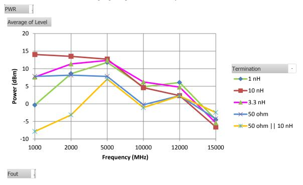
Let's start with the straight 50 ohm. We see flat power and then it starts to roll off. Recal that at 5 GHz, there is a dip in output impedance. After this, it is likely impacted by losses and parasitics. Now look at the 50 ohm  $\parallel$  10 nH. The basic idea here was to eliminate the DC drop across the resistor, but it only seemed to make things worse.
