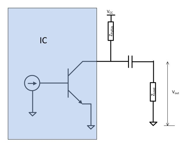
For high frequency, it also has several considerations. The choice and layout placement for the pull-up component is critical to output power and harmonics. Also, the assumption that the transistor output is high impedance is not necessarily true either. This paper attempts to bring some explanation to the behaviors of these open collector outputs through matching theoretical explanations to measured data.
