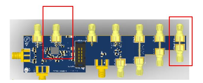
The loss of this board was measured over frequency and it was found to be about 0.2 dB. Although this board was not the dual PLL board (TIDA-01410), the PLL on it was a copy of this layout and therefore it can be assumed that the losses would be the same.
