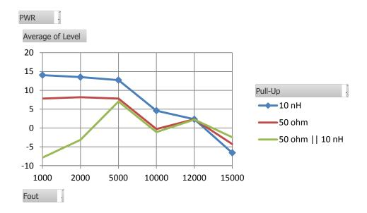
Now let's compare inductor to resistor. Around 1-5 GHz, the inductor impedance is high enough relative to the 50 ohm spectrum analyzer and we see 6 dB improvement. I think it's
