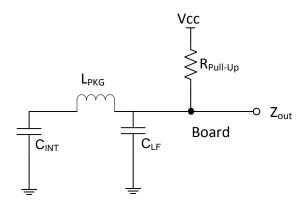
The above model was used to model the package impedance. Note that these are not exact values, but rather coarse estimates.
