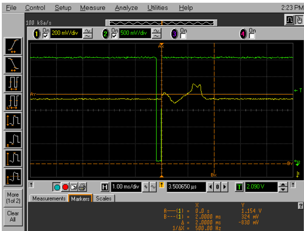
Figure 3 Pin 3 (VbiasVCO) Bias Time from Powerdown State (from Valid Lock) to POWERDOWN=0 with
