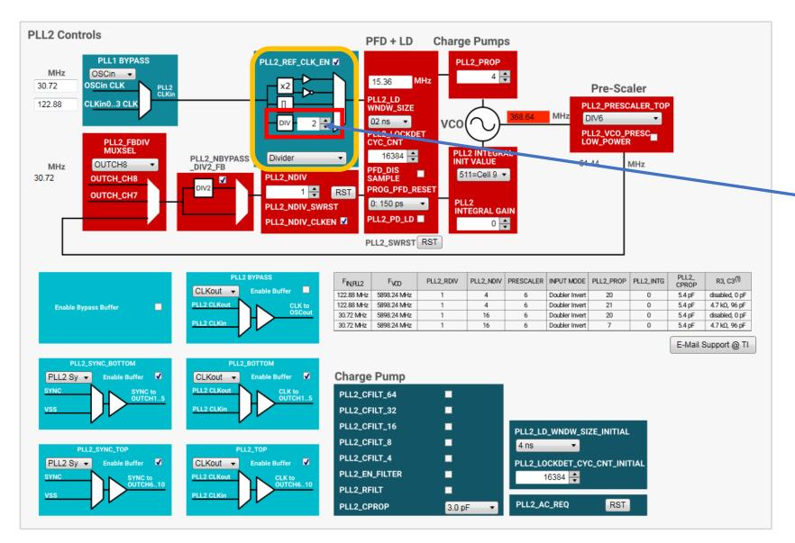
Case1. Increase setting value from 1 to 2. Case2. Decrease setting value from 3 to 2. PLL2 is locked at case1 and PLL2 is not locked at case2.
