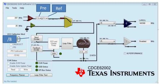
Frequency Planner generates 148.5MHz from 297MHz using the following parameters.
