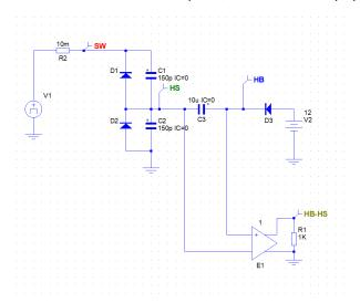
Simulated HS sensing circuit and C3 capacitor charging scheme in Simplis:
