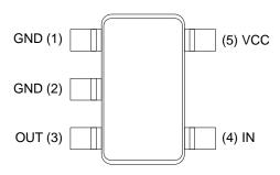
Figure 3. Pin Configuration (Top View)
