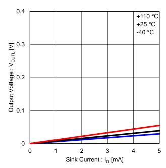
Figure 8. Output High Voltage
