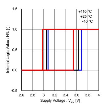
Figure 7. Under Voltage Lock Out
