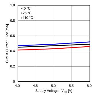
Figure 4. Operating Current (IN = 1kHz)
