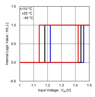
Figure 6. Input Threshold Voltage
