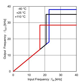
Figure 10. Output vs Input Frequency Characteristics (Low Frequency)
