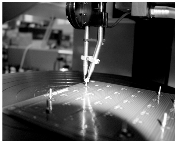
Figure 5. Pull Test Carried Out on the SMD 8 Bump (0.17 mm Diameter Bump)
