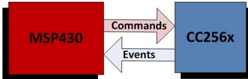
As shown in the diagram above, the host (MSP430) sends HCI commands to the controller (CC256x). The controller then sends HCI events to the host as a response to the HCI commands. All HCI commands follows this format for all packets:
