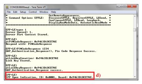
e) The two devices are now connected. Data can be sent/received from the two devices as shown here.
