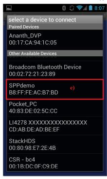
d) Select and Pair it with the device running the SPPdemo. If it needs a pincode enter a pincode on the app/phone. The MSP430 will prompt for a **PINCodeResponse**. Type **PINCodeResponse** < the pin code you used for the phone > in the prompt. It will pair and you should see an open indication on the MSP430.
