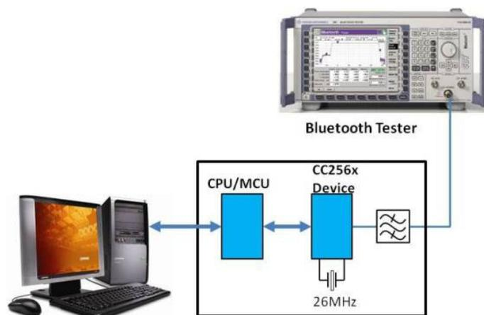
Figure: CC256x Bluetooth RF SIG mode test setup
