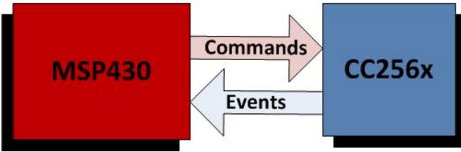
As shown in the diagram above, the host (MSP430) sends HCI commands to the controller (CC256x). The controller then sends HCI events to the host as a response to the HCI commands. All HCI commands follows this format for all packets:
