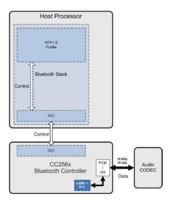
As shown in the diagram above WBS allows 16KHz sampling rate at the same air speed of 64kbps.
