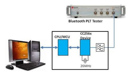
The VS HCI commands for the PLT test mode are below. See [HCI VS Commands (http://processors.wiki.ti.com/index.php/CC256x\_VS\_HCI\_Commands#HCI\_VS\_DRPb\_BER\_Mete r\_Start\_.28oxFD8B.29)] for more info on syntax.
