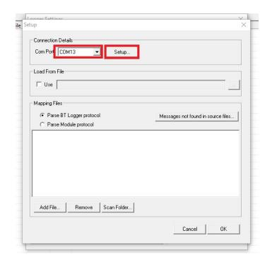
Note: Make sure the COM port number is less than 50. If not, change the COM port number to a lower value from the control panel. Reference (http://www.sealevel.com/support/article/AA-00441/0/How-to-change-asynchronous-serial-COM-port-assignments-in-Windows-Device-Manager.html)
