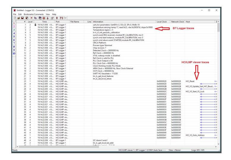
15. When all the relevant traces (BT Logger and HCI/LMP viewer) for the instance are captured, use File->Save As... to save the logs as a \*.lgr file.
