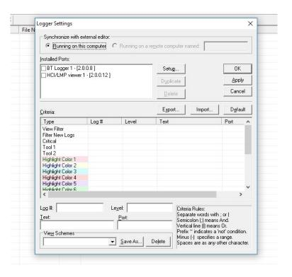
3. Select the BT Logger 1 under the Installed Ports list and click on Setup... button.
