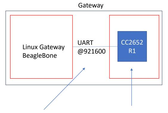
Probing UART Tx from CC2652RB shows same data loss as capturing UART data in Linux UART driver
