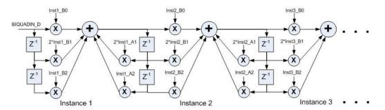
Note that the middle taps of the B and A coefficients are multiplied by 2 in the component. So, the coefficient values should be configured as ½ the original value.
