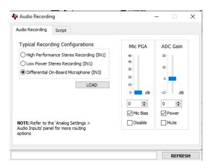
3. Set PGA Gain using Audio Inputs/Input Volume Control
