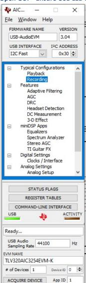
2. Open Recording Panel from Typical Configurations; select Differential On-Board Microphone; click LOAD to program Device.
