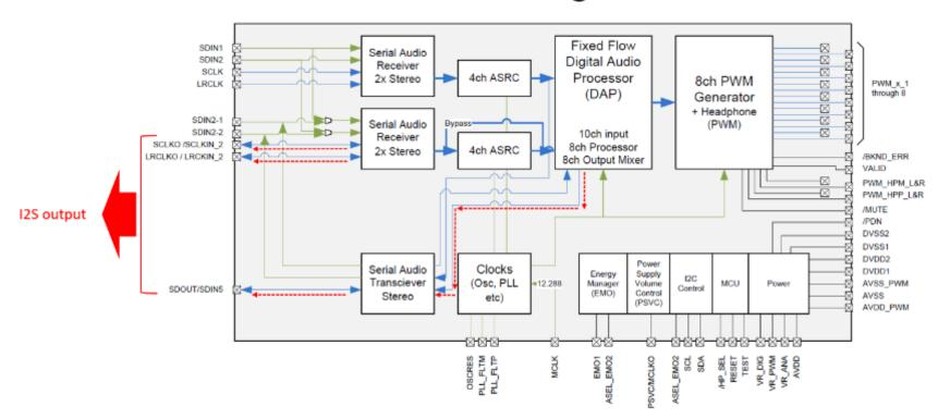
The customer is checking the combination of the TAS5548EVM replacing the IC with the TAS5558 and the PurePath Console 1.16, but the signal processed by DAP (Biquad Control/Tone/Volume/Loudness/DRC) is not output from the SDOUT.
