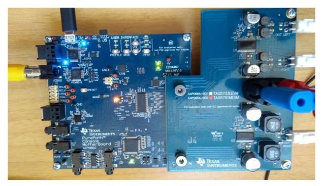
The boards are supplied with 24Vdc, USB to PC, coax SPDIF. User interface LEDs are not lit, the buttons are not working.
