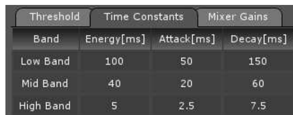
Figure 89. HF7 DRC Time Constants Tab for 3-Band Compressor
