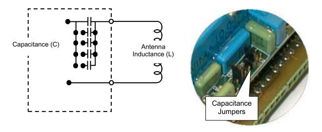
Figure 7. Capacitance Fine-Tuning
