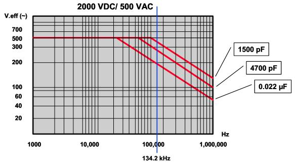
Figure 23. Polypropylene Capacitor De-rating
