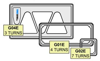
Figure 20. Windings Vs. Inductance
