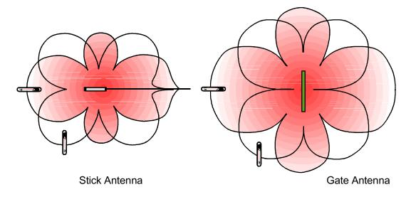
Figure 28. Antenna Field patterns
