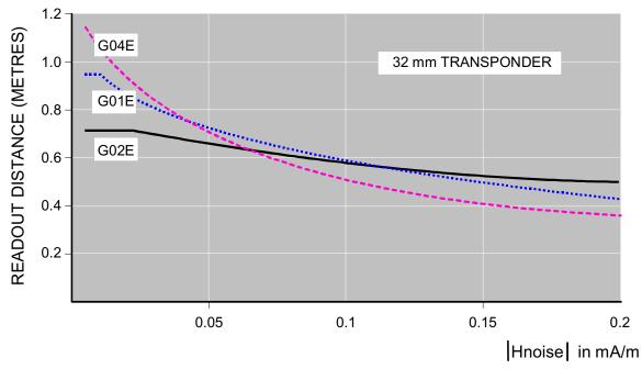
Figure 19. Reading Range Reduction due to Noise
