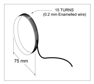
Figure 36. MicroReader Antenna 3
