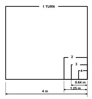
Figure 21. Single Loop Vs. 27 µH Inductance
