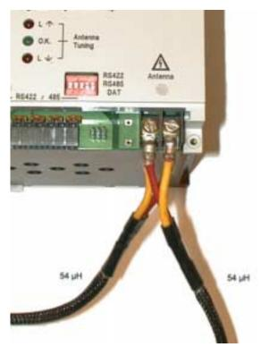
Figure 32. Two 54 µH Antennas connected in Parallel (out-of-phase)
