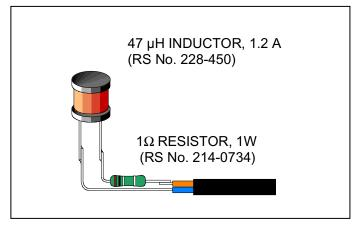
Figure 34. MicroReader Antenna 1
