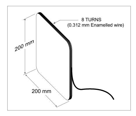
Figure 37. MicroReader Antenna 4
