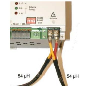
Figure 30. Two 54 µH Antennas Connected in Parallel (In-Phase)
