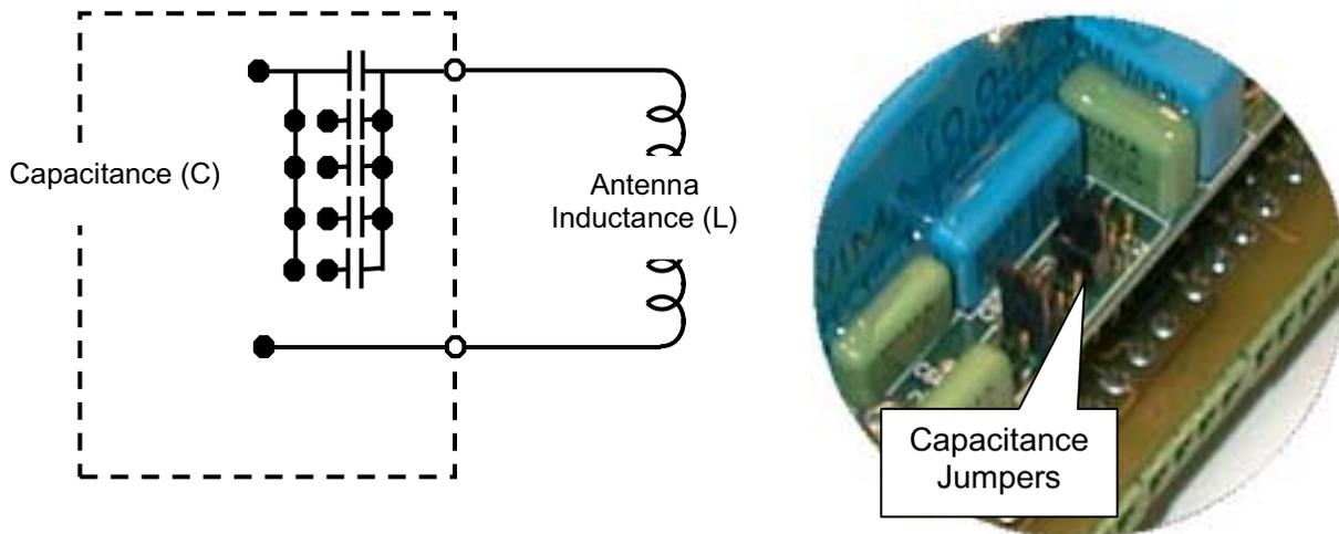
**Figure 7. Capacitance Fine-Tuning**
