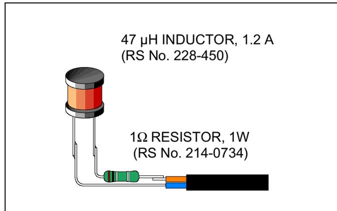
**Figure 34. MicroReader Antenna 1**
