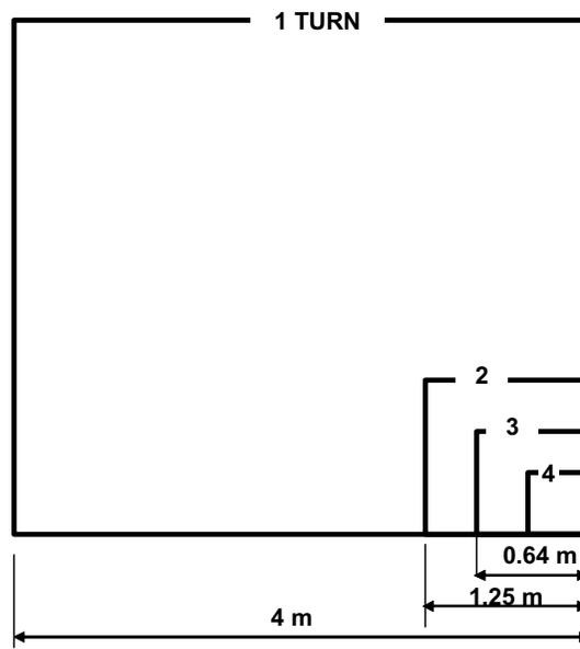
**Figure 21. Single Loop Vs. 27  $\mu$ H Inductance**
