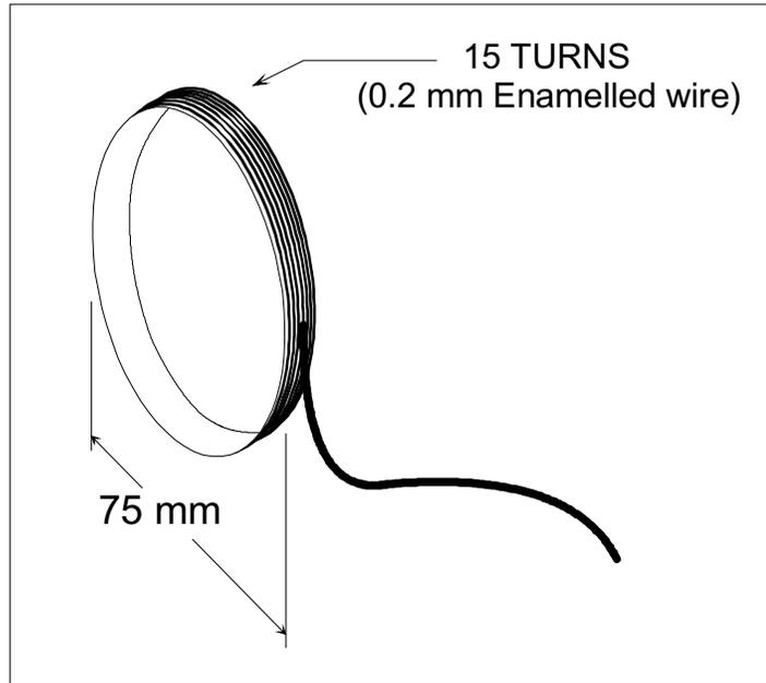
**Figure 36. MicroReader Antenna 3**
