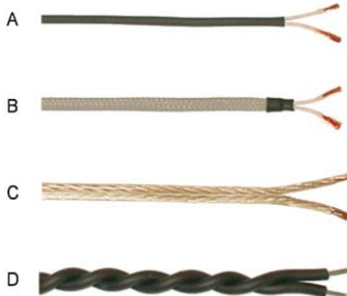
**Figure 25. Antenna Tail Construction**
