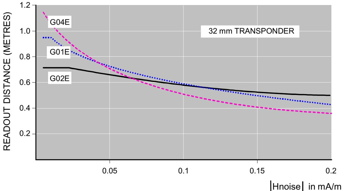
**Figure 19. Reading Range Reduction due to Noise**
