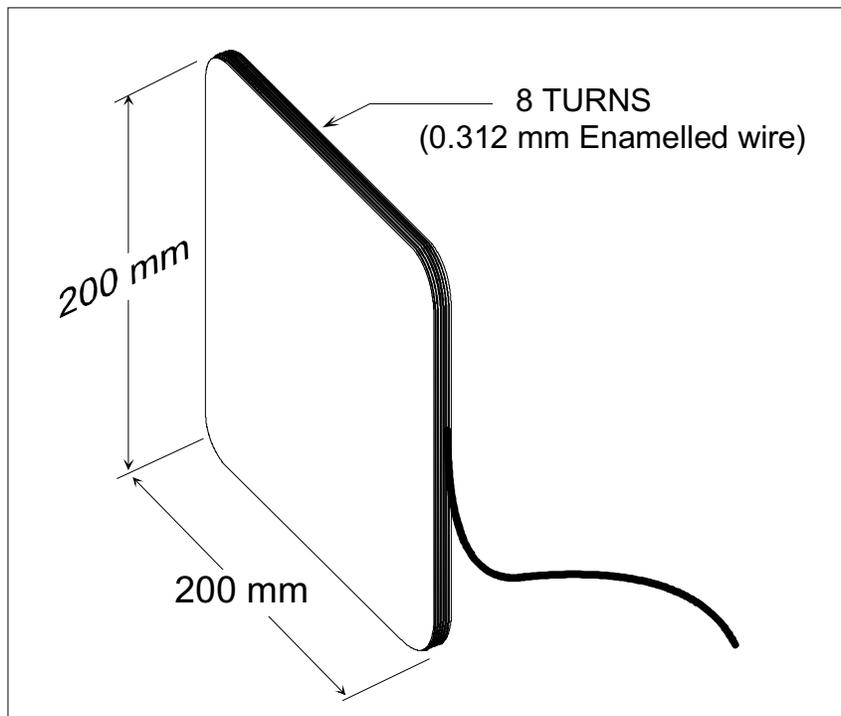
**Figure 37. MicroReader Antenna 4**
