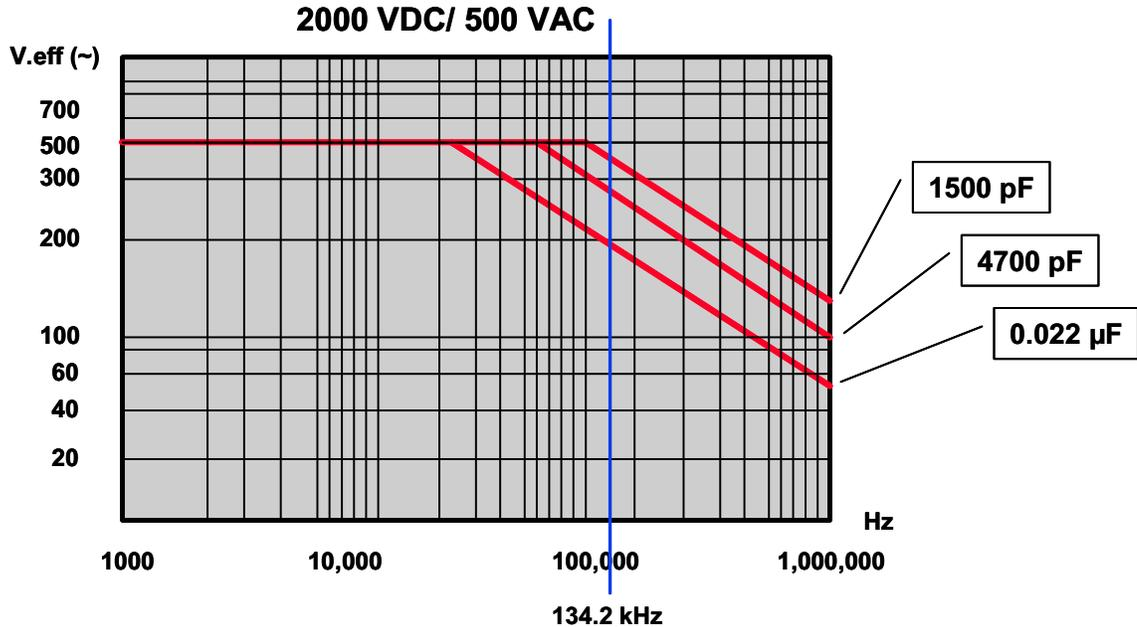
**Figure 23. Polypropylene Capacitor De-rating**
