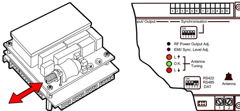
**Figure 22. Out of Tune Conditions**
