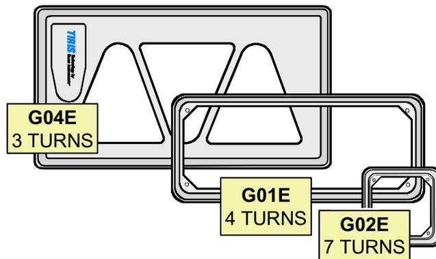
**Figure 20. Windings Vs. Inductance**
