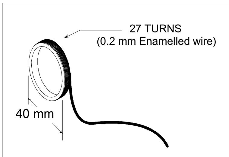
**Figure 35. MicroReader Antenna 2**
