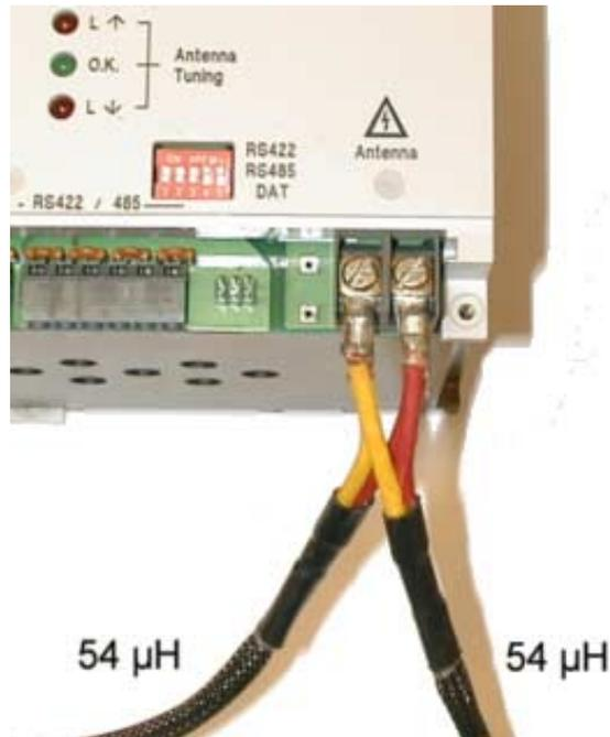
**Figure 30. Two 54  $\mu\text{H}$  Antennas Connected in Parallel (In-Phase)**
