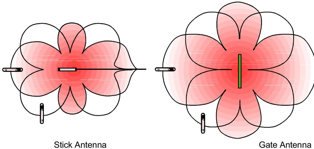
**Figure 28. Antenna Field patterns**
