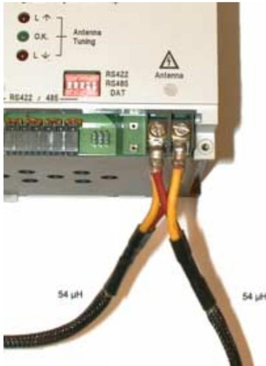
**Figure 32. Two 54  $\mu$ H Antennas connected in Parallel (out-of-phase)**
