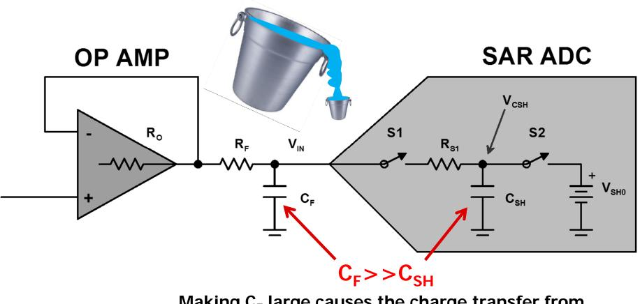
Making  $C_F$  large causes the charge transfer from  $C_F$  to  $C_{SH}$  to have minimal effect on  $C_F$  voltage
