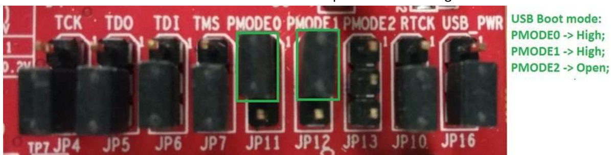
Figure 1 - PMODE Jumper settings for USB Boot Mode
