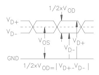
FIGURE 3. LVDS output signal levels.
