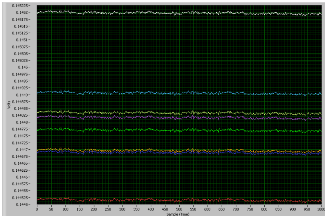
Figure 33. Eight-Channel Read of Internal Temperature
