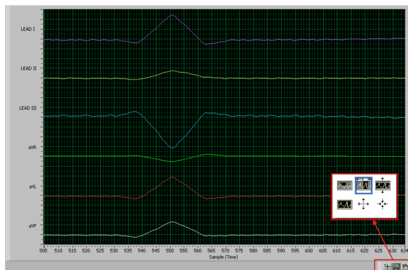
Figure 28. ECG Signal Zoom Feature for Six Leads
