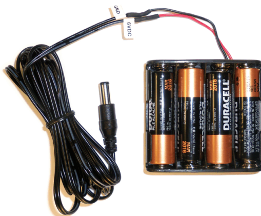
Figure 49. Recommended Power Supply for ADS1x98ECG-FE
