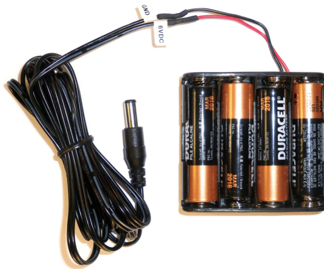
Figure 52. Recommended Power Supply for ADS1298R
