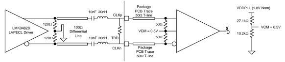
The AC coupled network requires series capacitors to allow the common mode voltage on both the SYSREF driver and SYSREF receiver to establish independently. Therefore, the series capacitors, along with the DAC3xJ8x SYSREF receiver on-chip 50ohm termination, forms a high pass response to isolate the common mode voltage of the driver and receiver. The high pass corner is the typical first order response with cut-off frequency and time constant as follow:
