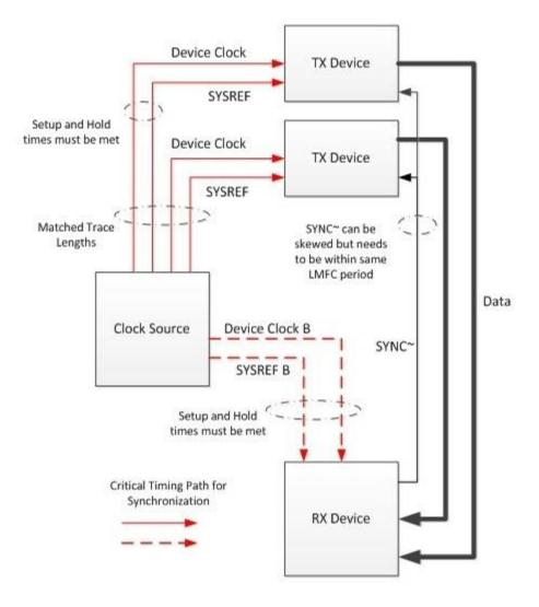
Figure 2: Subclass 1 timing signals with trace length matched SYSREF and device clock groups (copy from Blogpost <u>https://e2e.ti.com/blogs\_/b/analogwire/archive/2014/10/24/jesd204b-</u> <u>understanding-subclasses-part-1</u>)
