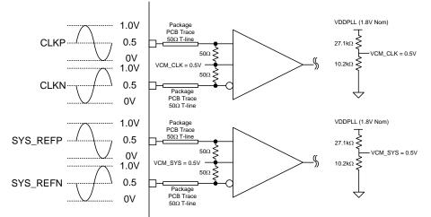
The DAC3xJ8x DACCLK and SYSREF receivers have delay matched receiver design given the external clock and SYSREF inputs have identical driver behavior and are AC coupled. The internal resistor divider networks set the common mode voltage of the DACCLK and SYSREF receivers at 0.5V nominal.
