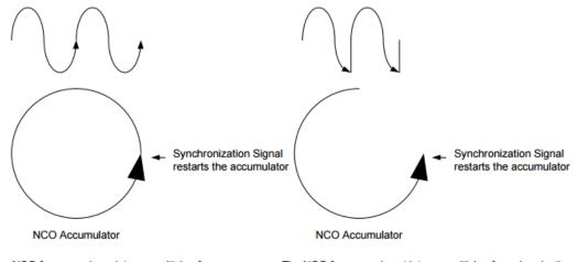
The NCO frequency is an integer multiple of the synchronization signal. The NCO can cycle through completely before the next reset. The NCO frequency is not integer multiple of synchronization signal. The NCO cannot cycle through completely before the next reset. Output waveforms are distorted.
