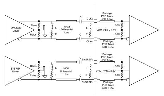
Moreover, both the DACCLK and SYSREF receiver path may have such implementation to form a part of a matched bandpass network. The PCB layout of both paths may be matched, but the exact bandpass frequency and components may not match since the DACCLK is usually a much higher frequency than SYSREF. This may be an option if the DACCLK port is being used as a slow reference clock for the DAC3xJ8x on-chip PLL path.
