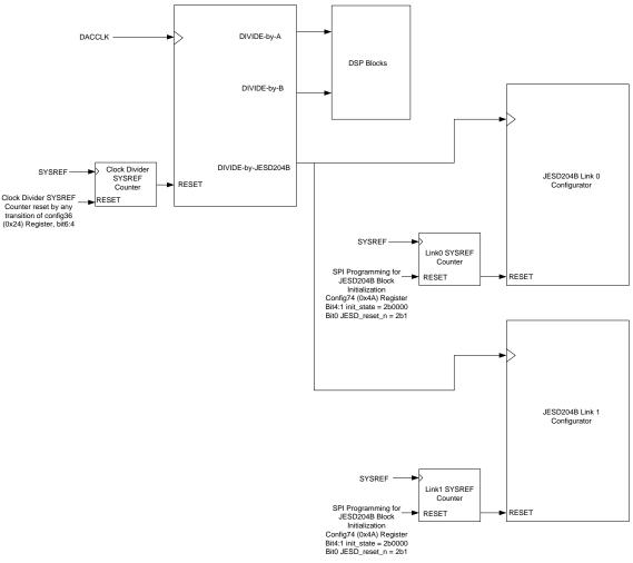
Figure 1. Clock Divider and JESD204B Simplified Circuit Diagrams
