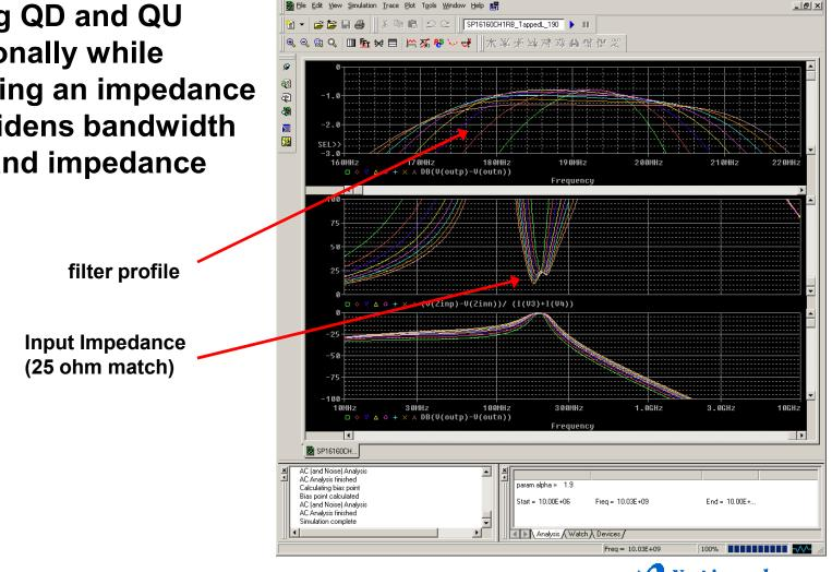
SP16160CH1R8 TappedL\_190MHz - OrCAD PSpice A/D Demo - [SP16160CH1R8 TappedL\_190MHz.dat (active)
