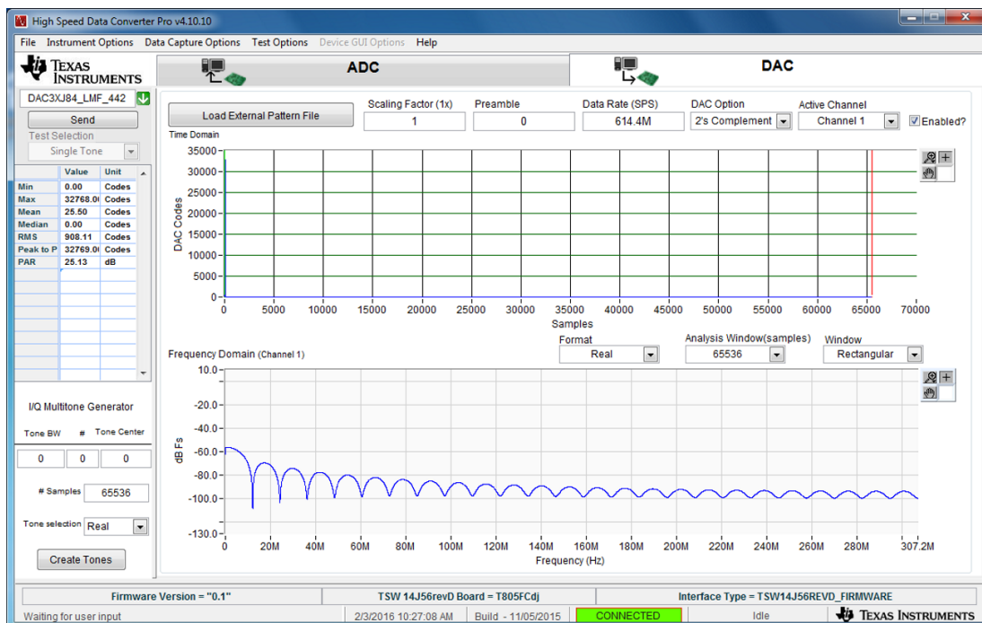
Figure 22. HSDC PRO GUI DAC Settings and Pattern File Loading
