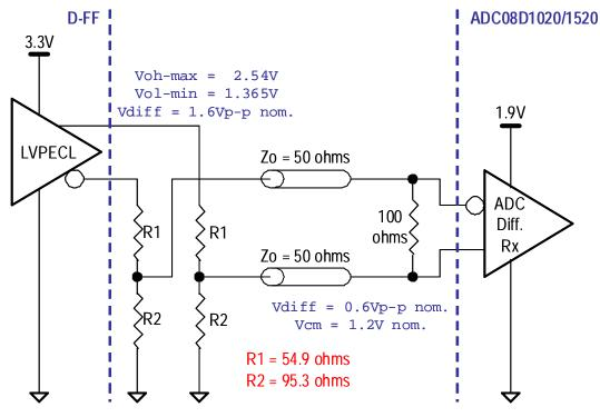
Figure 6 – PECL to ADC08D1020/1520's "LVDS-Like" Differential Input
