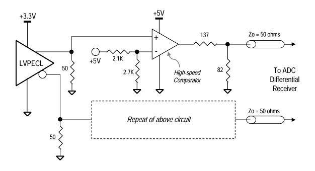
Figure 5 – Conceptual LVPECL-to-CMOS level translation circuit
