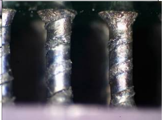
Figure H. The image of the contacts between the column and PCB board showed no anomalies on SN21.
