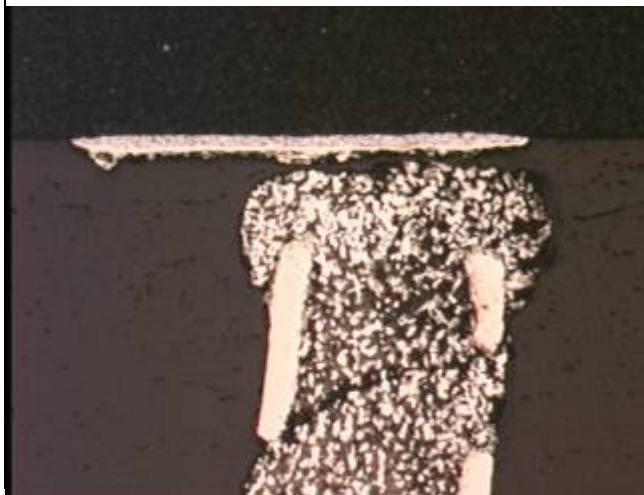
Figure II. High magnification photo of the first contact between the column and pad of the package on SN29.
