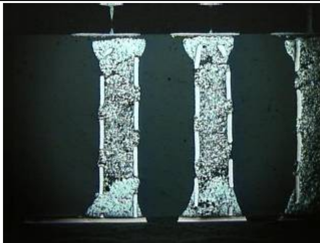
Figure O. High magnification photo of the first contact between the column and pad of the package on SN3.
