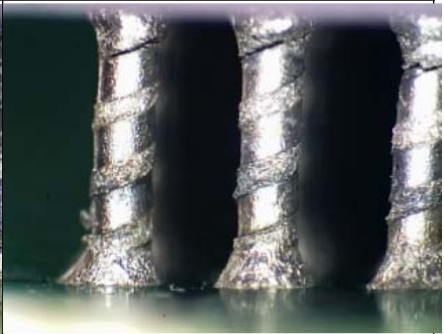
Figure C. The image of the contacts between the column and PCB board showed no anomalies on SN15.
