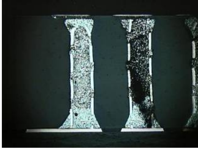
Figure EE. High magnification photo of the first contact between the column and pad of the package on SN27.
