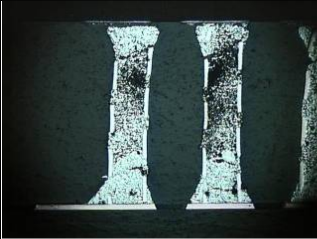
Figure S. High magnification photo of the first contact between the column and pad of the package on SN15.
