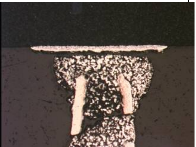
Figure JJ. High magnification photo of the second contact between the column and pad of the package on SN29.
