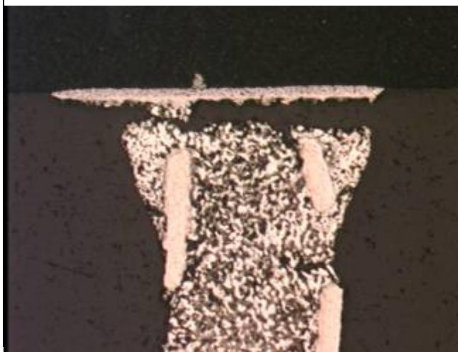
Figure MM. High magnification photo of the seventh contact between the column and pad of the package on SN29.
