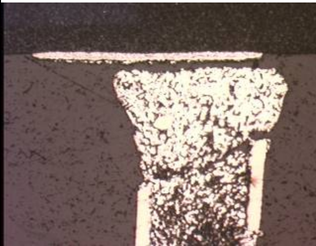
Figure S. High magnification photo of the first contact between the column and pad of the package on SN15.
