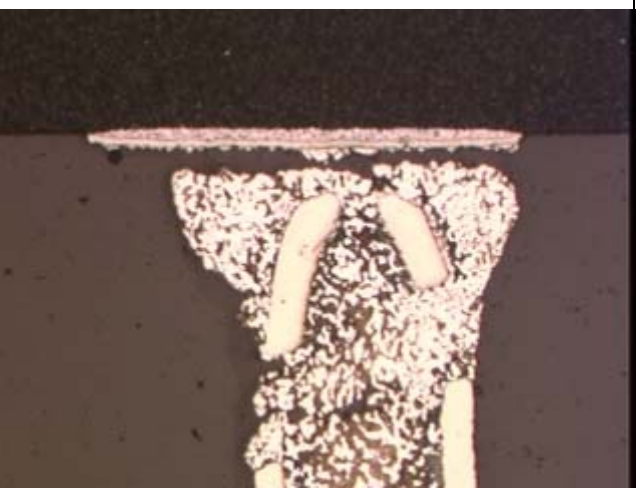
Figure X. High magnification photo of the second contact between the column and pad of the package on SN21.
