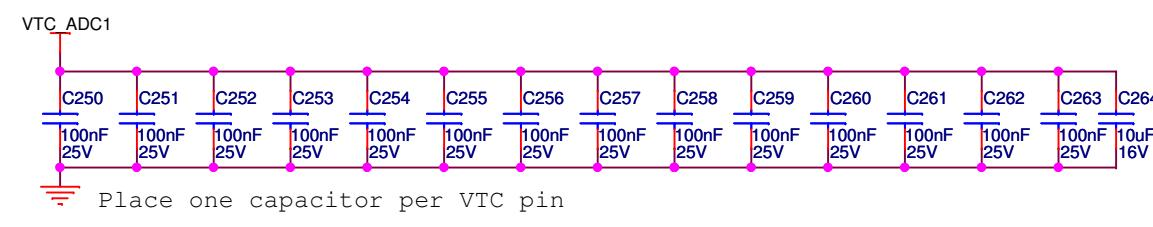
Place one capacitor per VTC pin
