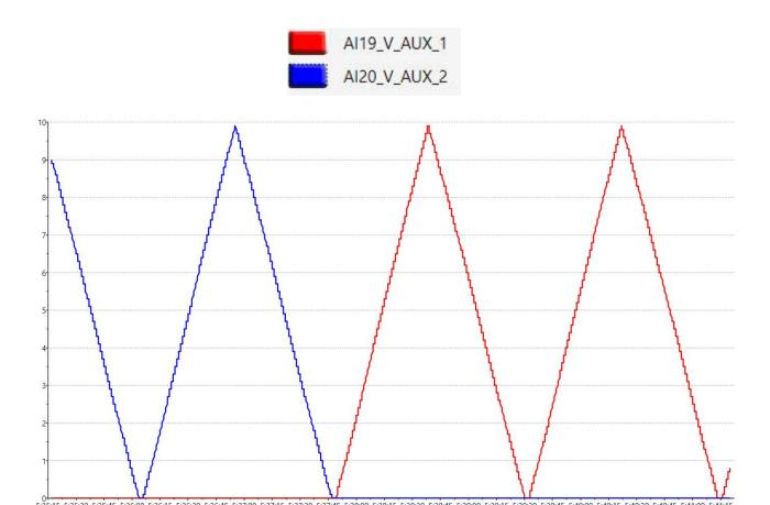
Sweep 0-10V on ADC2 and ADC1 floating.
