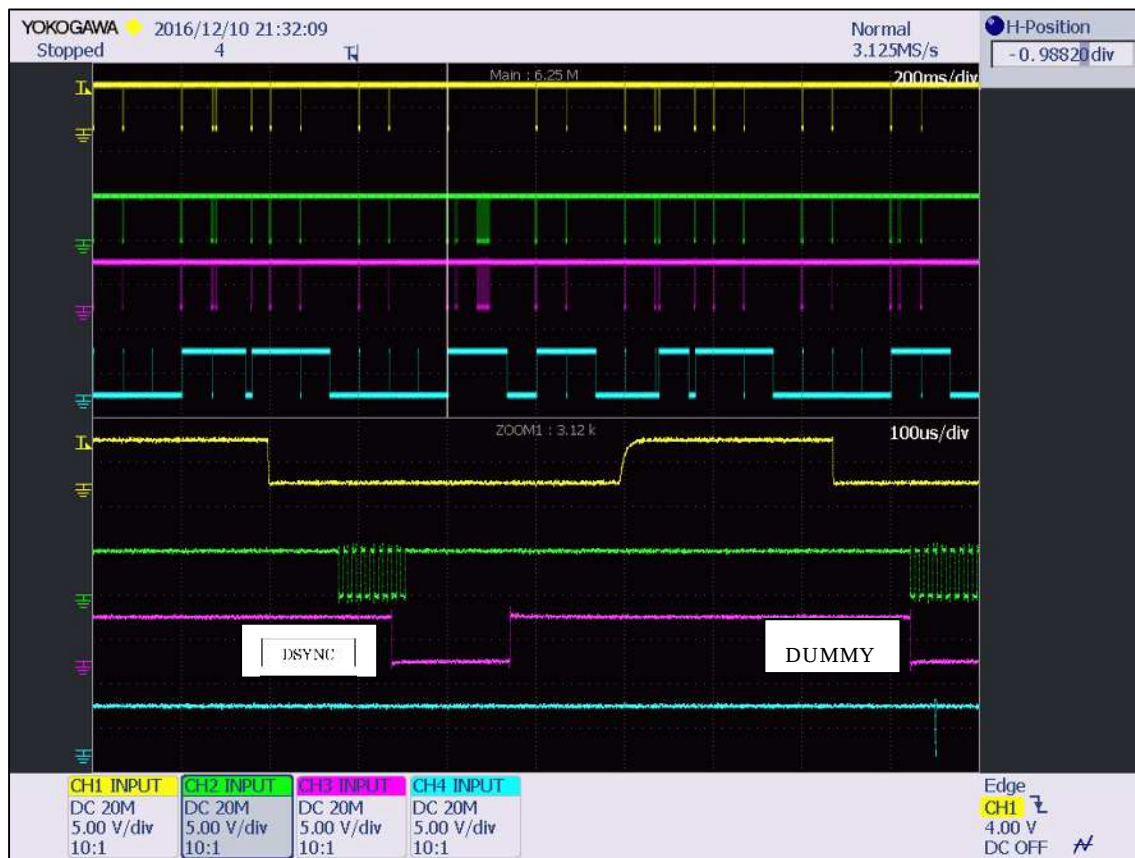
Figure.4 DSYNC command and DUMMY command (Yellow:CS Green:CLK Pink:DIN Blue:DRDY)
