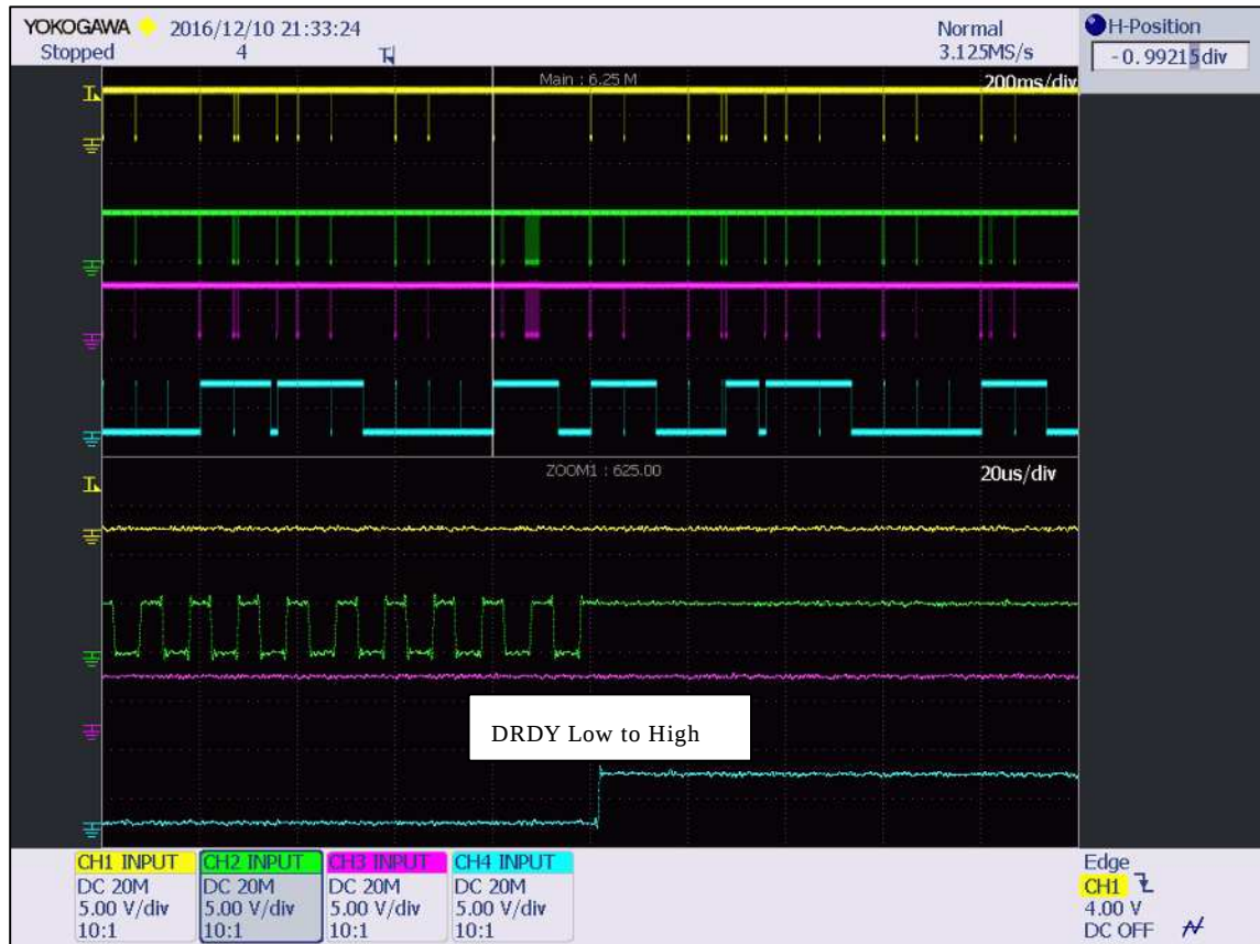
Figure.3 Zoomed DRDY High timing on measurement data reading (3) (Yellow:CS Green:CLK Pink:DIN Blue:DRDY)
