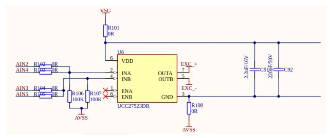
Using 2 wire mode, we are desoldering R103 and R105, leaving connected only AIN2 / AIN3
