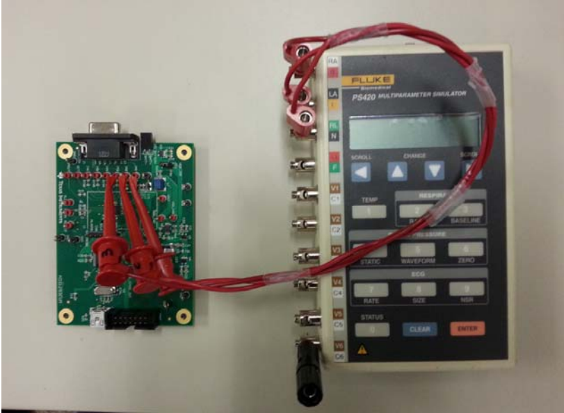
Figure 2. Homemade cable connected to the input TP connectors for testing the evaluation board using an ECG emulator
