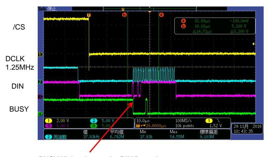
BUSY High to Low at the DIN first pulse Is this a correct spec?
