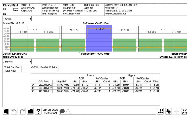
Figure 425. TX 20-MHz LTE Output Spectrum at 1.8425 GHz
