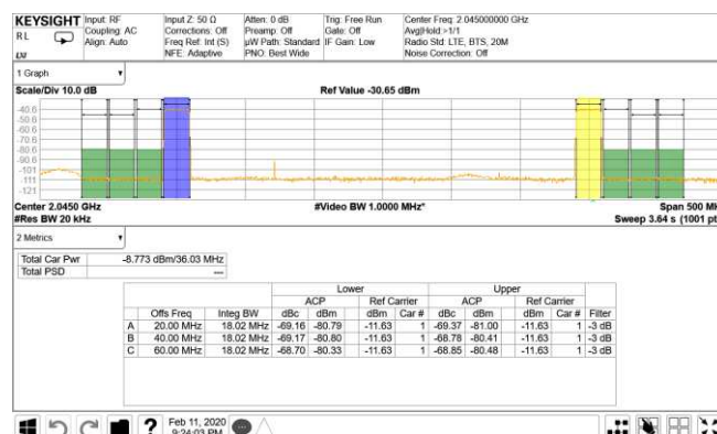
Figure 606. Band 1 + Band 3 Output Spectrum With Two-Carrier LTE Signals
