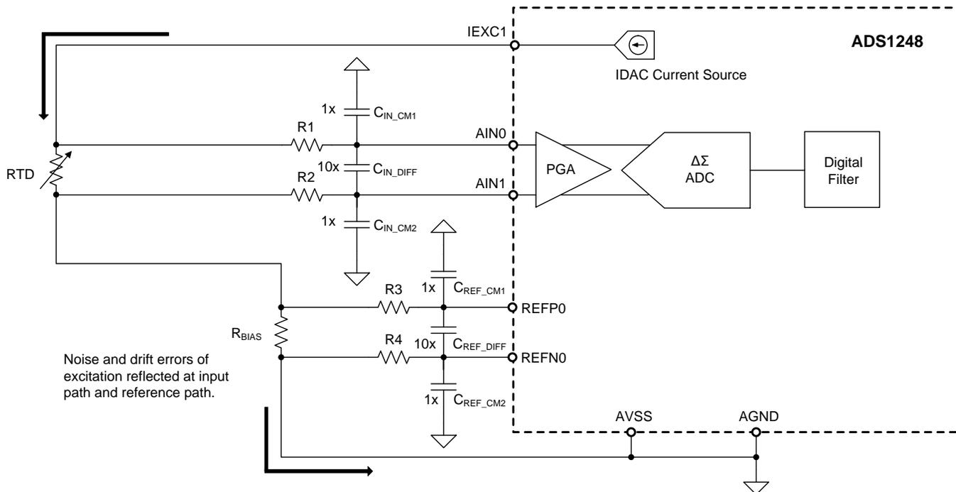
**Figure 3. Four-Wire Ratiometric RTD Measurement with Filters ( $R_{LEAD}$  Removed for Simplicity)**
