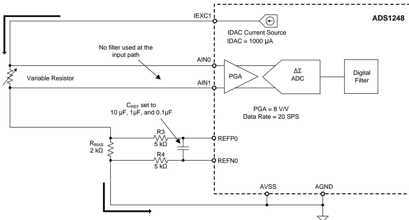
Figure 6. Circuit for Noise Measurement Experiment with Mismatched RC Filters
