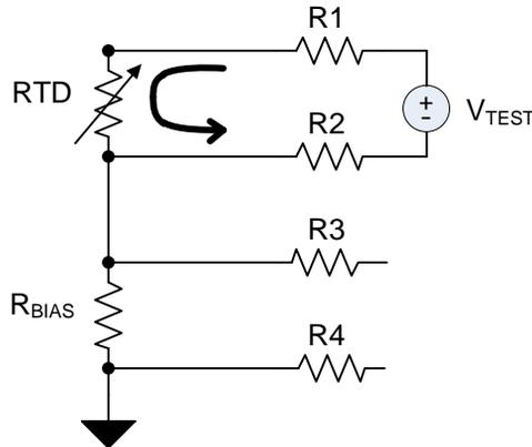
Figure 4. Simplified RC Circuit to Find the Corner Frequency of the Differential-Mode Input Filter
