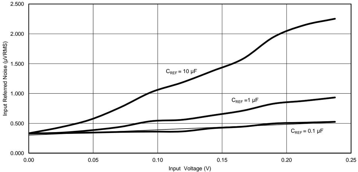
**Figure 7. Input Referred Noise vs Input Voltage Using Mismatched RC Filters**
