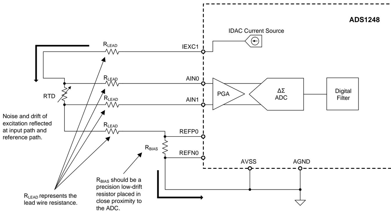
**Figure 1. Four-Wire Ratiometric RTD Measurement Using the ADS1248**
