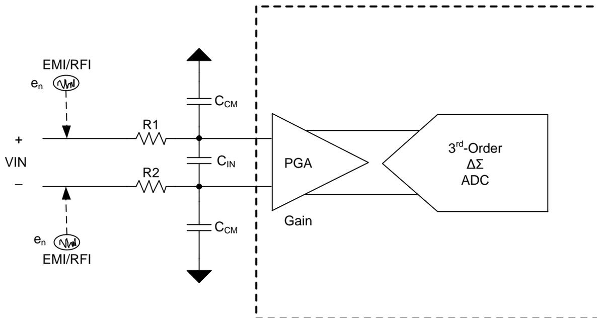
Figure 2. Typical Differential and Common-Mode Filter
