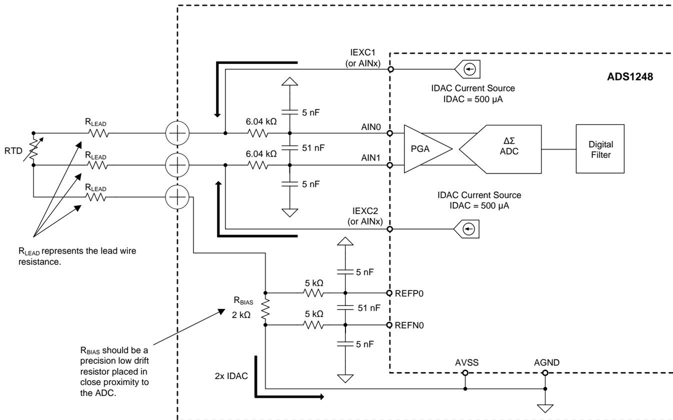
Figure 10. Example of a Three-Wire Ratiometric Configuration with RC Filters
