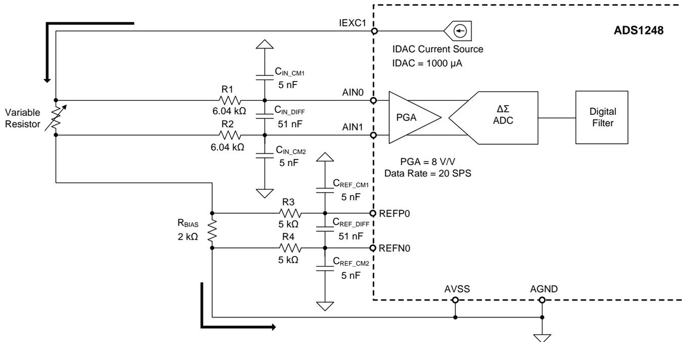
Figure 8. Example of a Four-Wire Ratiometric Configuration with RC Filters ( $R_{Lead}$  Removed for Simplicity)
