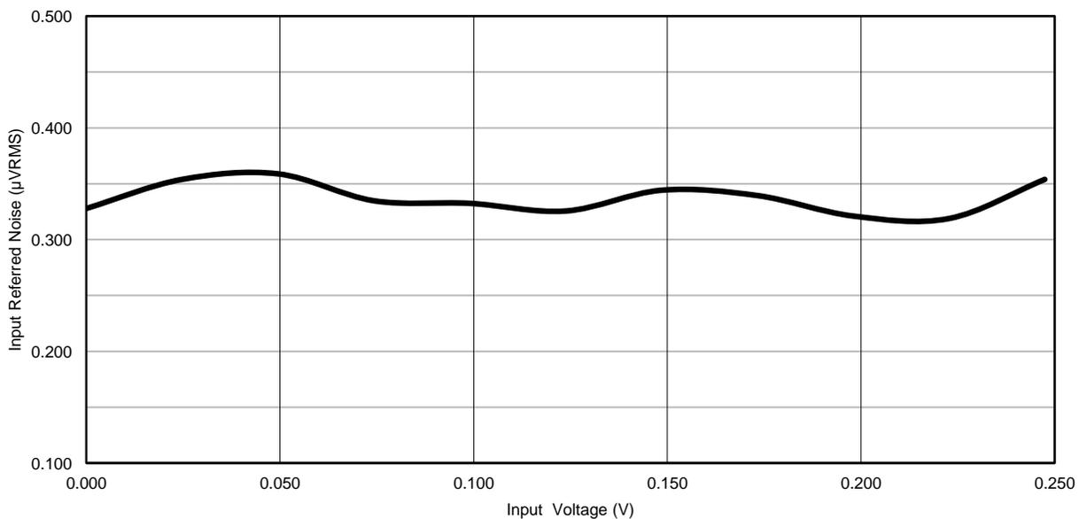
**Figure 9. Input-Referred Noise vs Input Voltage Using Matched RC Filters**
