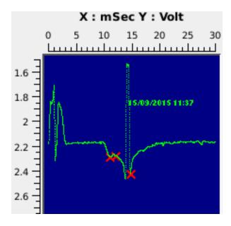
To confirm, we have applied 1.05v signal from function generator. In that case also waveform is displayed in the clipped form at 2.5v and clipped portion is displayed from 1.5v onwards as shown below.
