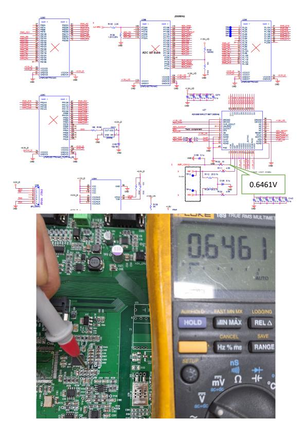
Delete R111, R124, R123,C144,C145,FPGA The measured VCM of the ADC is 0.6461V
