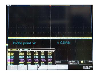
Voltage waveform of the ADS7828 analog input pin (Measured waveforms when the LM60CIM output is physically disconnected from the ADS7828 analog input pin during abnormal temperature indication)
