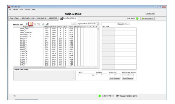
Once it is successful, go to ADC14DJ1350 tab, and in the "Top" subtab type in 1000 for the "F\_ADC\_FUNC" variable. After doing this, please click on the PLL0\_lock and PLL1\_lock signals below on the same page to make sue the clock has been locked. (This step can be skipped if the normal sine wave input signal is to be captured).
