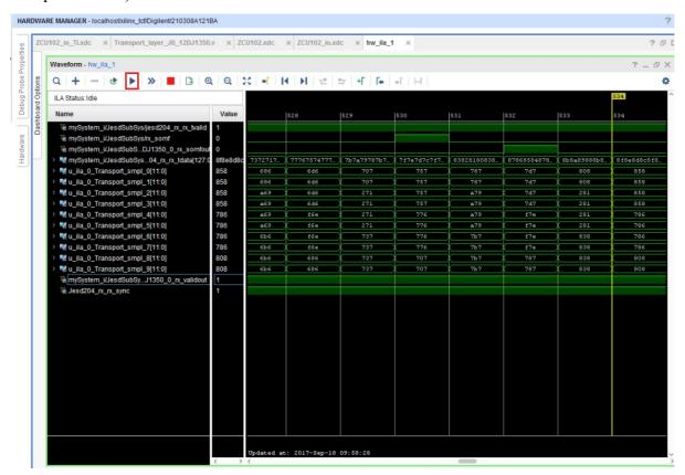
The **Jesd204\_rx\_rx\_tdata** can be grouped into 4 lanes of 32 bits each. This will make viewing much easier. This can be done by selecting the required signals (select 0 to 31 for lane0, 32 to 63 for lane\_1 etc.,) and right-clicking and selecting "**New Virtual bus**". Then name the new bus. After grouping into 4 lanes you will get something similar to the image below.
