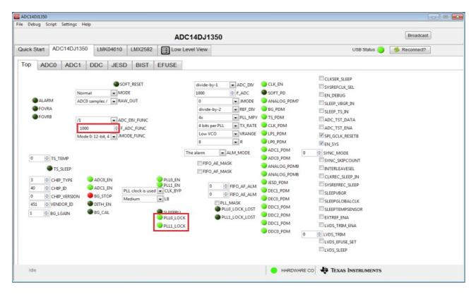
• Finally go the JESD subtab and set the "JTest" variable to **Ramp test mode.** This will enable the device to send a separate byte ramp on each lane.(This step can be skipped if the normal sine wave input signal is to be captured).
