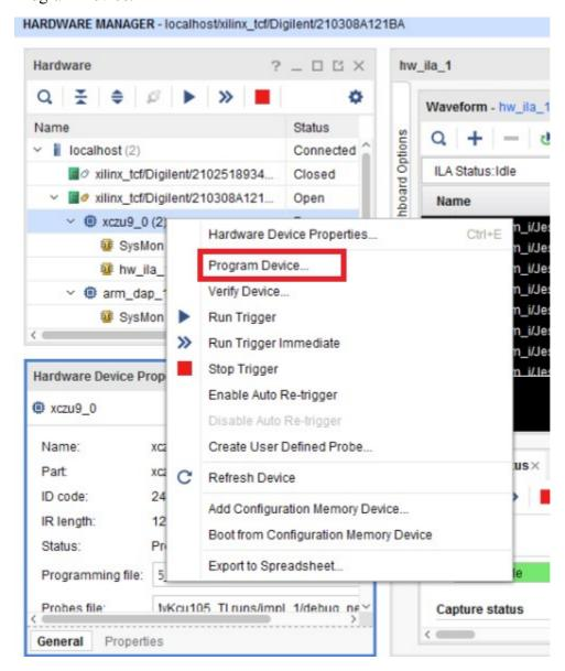
In the Pop-up. Select the "mySystem\_wrapper.bit" generated earlier in the Bitstream file path. In the Debug Probes file path mention the "debug\_nets.ltx" file which was also previously generated. Then press "Program".
