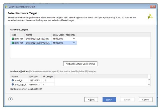
6) After that Right click on the ZCU102 device part number that is listed and press on Program Device.
