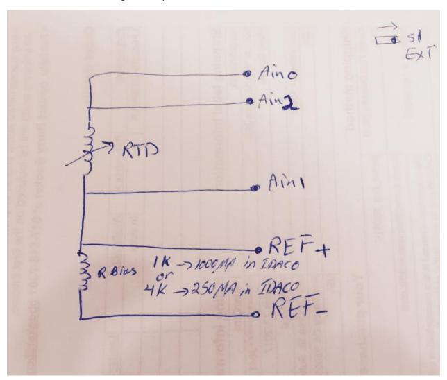
Please note I put 100 ohm resistor for RTD and 4 Kohm resistor for Rbias.
