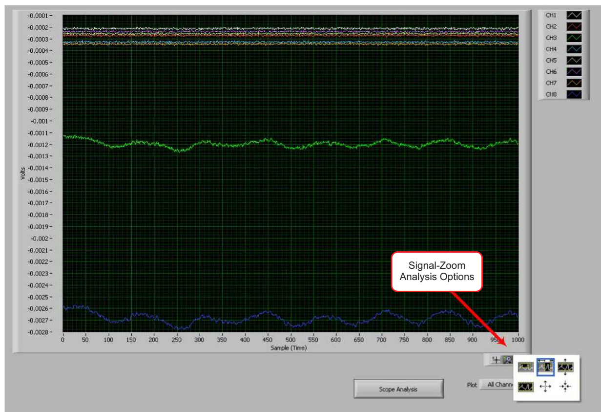
Figure 24. Zoom Option on the Waveform Examination Tool
