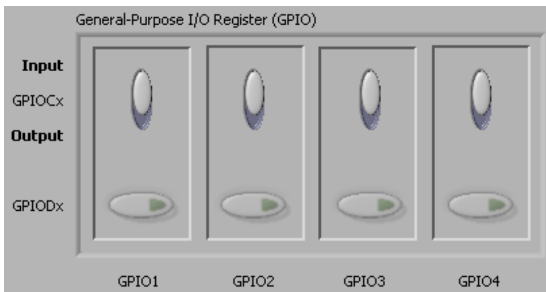
Figure 19. GPIO Control Register GUI Panel
