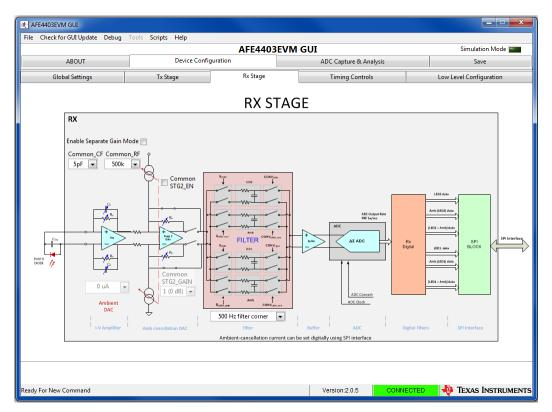
Figure 25. AFE4403: Device Configuration: Rx Stage
