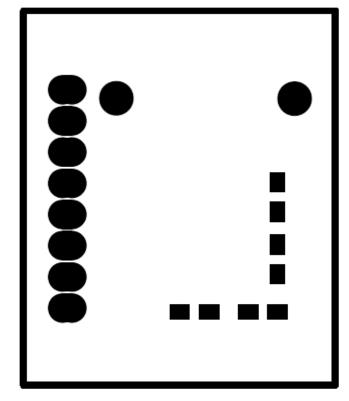
Figure 77. SFH7050 Sensor Board Bottom Solder Mask
