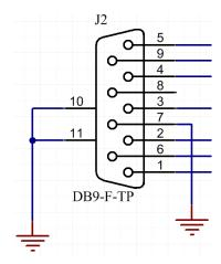
Figure 39. DB9 Pulse Oximeter Connector Pin Outs
