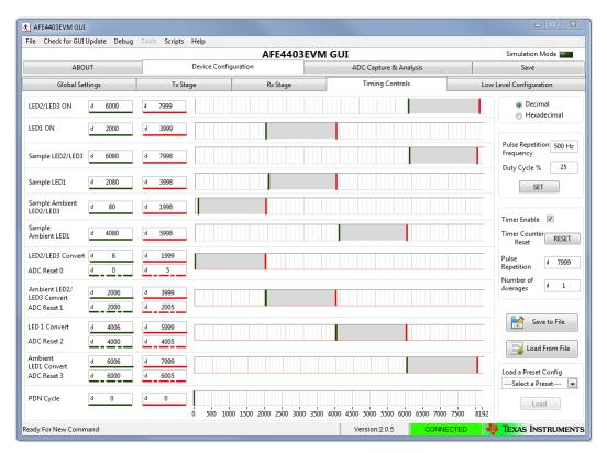
Figure 26. AFE4403: Device Configuration: Timing Controls
