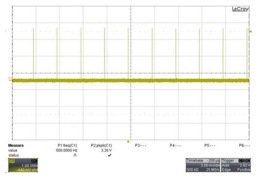
Figure 47. ADC RDY Waveform at 500-Hz PRF
