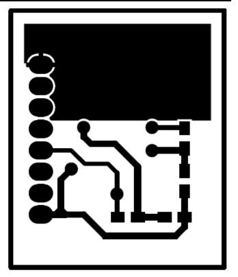
Figure 76. SFH7050 Sensor Board Bottom Copper
