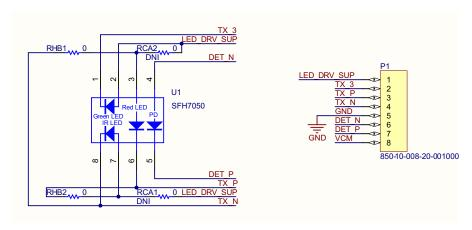
Figure 89. SFH7050 Sensor Board Schematic
