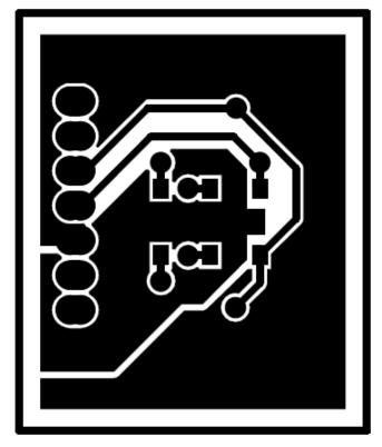
Figure 81. NJL5310R Sensor Board Top Copper
