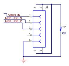
Figure 40. USB Micro Connector Pin Outs
