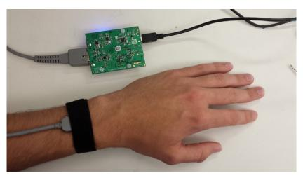
Figure 45. Setup for Obtaining Measurements from the Wrist
