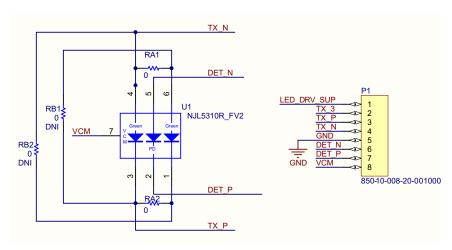
Figure 90. NJL5310R Sensor Board Schematic
