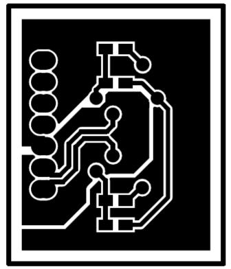
Figure 82. NJL5310R Sensor Board Bottom Copper
