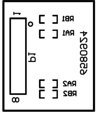
Figure 84. NJL5310R Sensor Board Bottom Silk Screen
