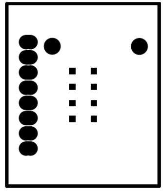
Figure 73. SFH7050 Sensor Board Top Silk Screen
