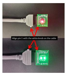
Figure 44. Sensor Board Cable Connections
