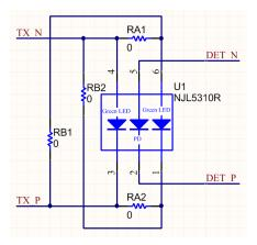
Figure 42. NJRC NJL5310R Sensor Board LED Connections
