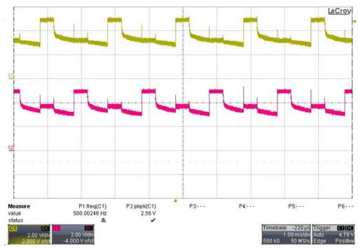
Figure 49. TXP and TXN After Connecting the Pulse Oximeter Cable
