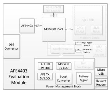
Figure 31. AFE4403EVM Block Diagram
