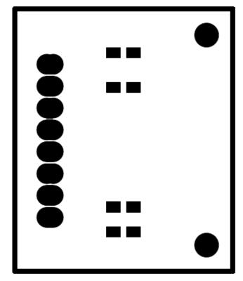
Figure 83. NJL5310R Sensor Board Bottom Solder Mask
