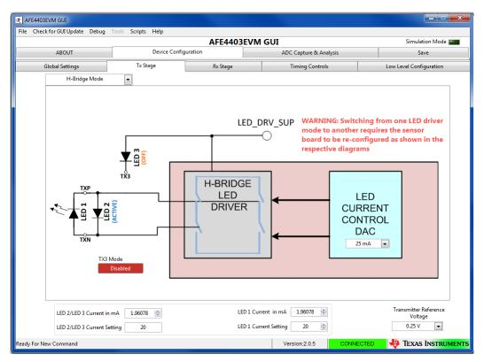
Figure 24. AFE4403: Device Configuration: Tx Stage
