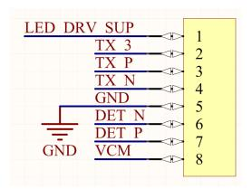
Figure 41. 8-Pin Connector
